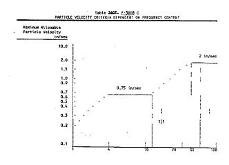
Blast Vibration Frequency, Hz
