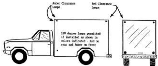
If equipped with three red identification lamps, the required clearance lamps may be mounted at any height so long as they indicate, as nearly as practicable, the extreme width of the vehicle.
