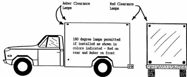
If equipped with three red identification lamps, the required clearance lamps may be mounted at any height so long as they indicate, as nearly as practicable, the extreme width of the vehicle.
