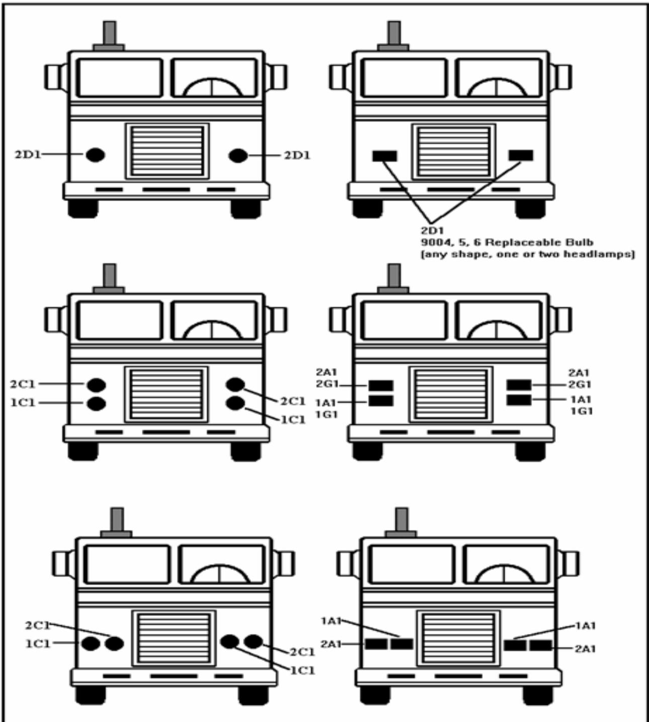
NOTE: ALWAYS inspect the following sealed beam and replacement bulb headlamps on LOW BEAM only:
