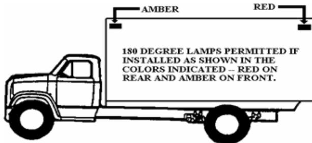
If equipped with three red identification lamps, the required clearance lamps may be mounted at any height so long as they indicate, as nearly as practicable, the extreme width of the vehicle.
