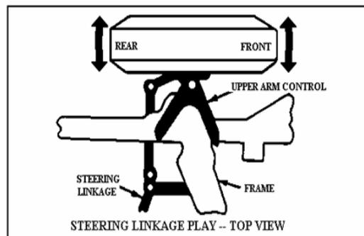
NOTE: With vehicle lifted properly, grasp tire at top and bottom, rock in and out and record movement. Wheel bearing looseness is detected by the relative movement between the brake drum or disc and the braking plate or splash shield.
