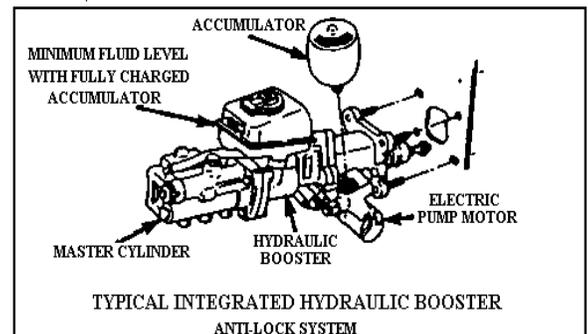
5. Condition of integrated hydraulic booster/anti-lock system with electronic pump. With the system fully charged, inspect system for fluid level and leaks.
