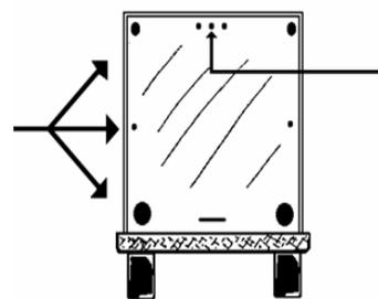
NOTE: Must be equipped with three red identification lamps
