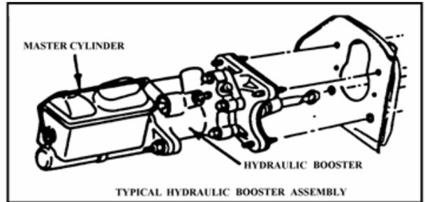
3. Condition of hydraulic booster power brake system. Inspect system for fluid level and leaks.
