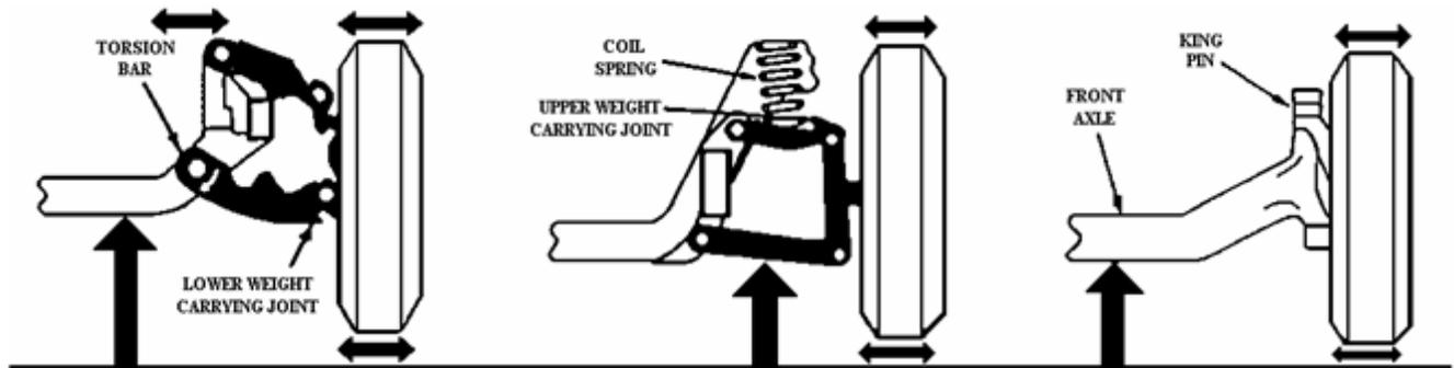
Proper lifting for wheel bearing, steering linkage looseness, and king pin play action
