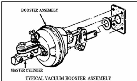
7. Condition of vacuum booster power brake system. Reject vehicle if there are collapsed, cracked, broken, badly chafed or improperly supported hoses and tubes, loose or broken hose clamps.
